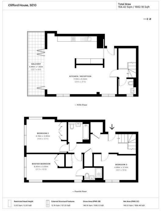
Spec floor plan captured for JLL, Greenwich on 19/03/2018 using 54,515,913 laser scan points, accurate to \*/- 3cm, Produced in accordance with Royal Institution of Chartered Surveyors Property Measurement Standards, incorporating International Property Measurement Standard (IPMS). If you intend to rely on any measurement in a transaction you should perform your own checks. Plot/Gardens illustrative only and excluded from all area calculations. Specific Sbace31bd5ee10c552c4des
