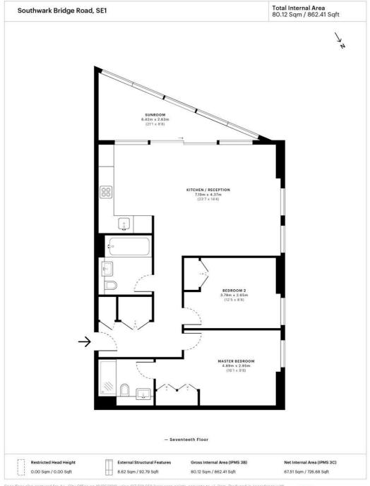
Spec floor plan captured for JLL, City Office on 18/06/2018 using 137,691,658 laser scan points, accurate to \*/- 3cm. Produced in accordance with Royal Institution of Chartered Surveyors Property Measurement Standards, incorporating International Property Measurement Standard (IPMS), if you intend to rely on any measurement in a transaction you should perform your own checks. Plot/Gardens illustrative only and excluded from all are calculations.
