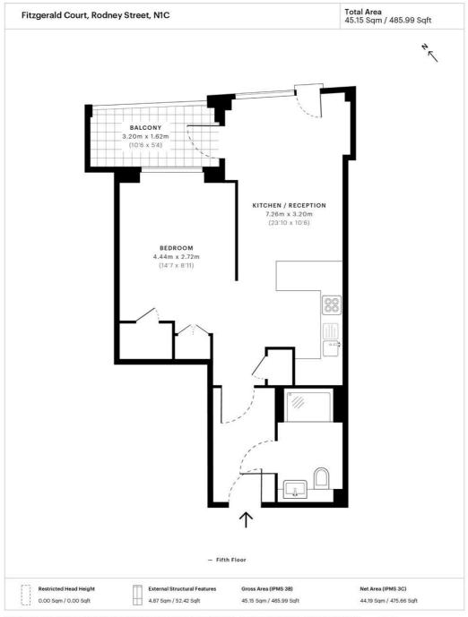
Spec floor plan captured for JLL, City Office on 15/08/2018 using 116,498,822 laser scan points, accurate to \*/- 3cm. Produced in accordance with Royal Institution of Chartered Surveyors Property Measurement Standards, incorporating International Property Measurement Standard (IPMS). If you intend to rely on any measurement in a transaction you should perform your own checks. Plot/Gardens illustrative only and excluded from all area calculations. SpeciD:5b7i90fa0315570c510557aa
