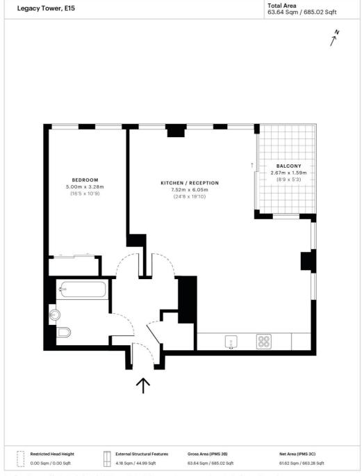
Spec floor plan captured for JLL, Stratford on 24/08/2018 using 137,541,341 laser scan points, accurate to +/- 3cm. Produced in accordance with Royal Institution of Chartered Surveyors Property Measurement Standards, incorporating International Property Measurement Standard (IPMS). If you intend to rely on any measurement in a transaction you should perform your own checks. Plot/Gardens illustrative only and excluded from all area calculations. SpeciD: 557e7687f83980c79897709
