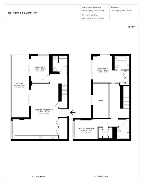
This floor plan was captured for JLL, knightsbridge on 12/03/2018. Architectural features to scale, derived from millions of laser scan points, accurate to +/- 3cm and produced in accordance with the Royal Institute of Chartered Surveyors Property Measurement standards. Gross Internal Area is measured from the internal faces of external walls and includes internal walls/obstructions. Net Internal Area excludes internal walls/obstructions. Net Internal Area is under the property of the prop
