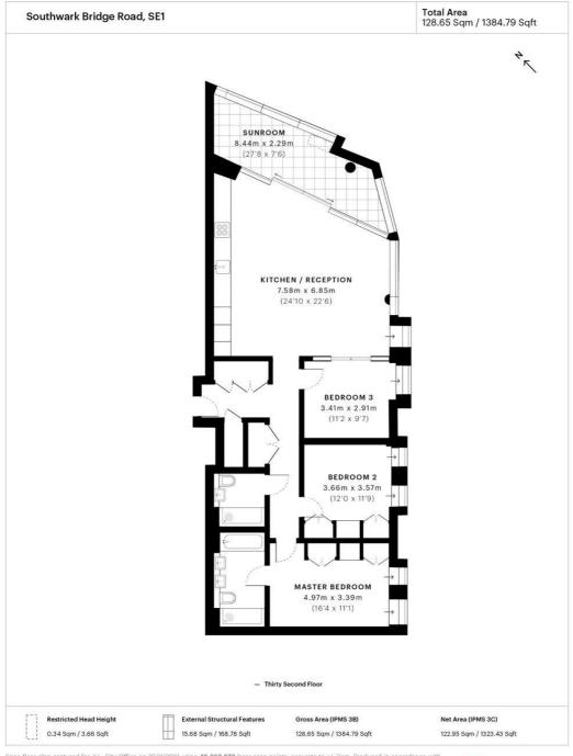
Spec floor plan captured for JLL, City Office on 29/11/2018 using 42,363,273 laser scan points, accurate to \*/- 3cm. Produced in accordance with Royal Institution of Chartered Surveyors Property Measurement Standards, incorporating International Property Measurement Standard (IPMS). If you intend to rely on any measurement in a transaction you should perform your own checks. Plot/Gardens illustrative only and excluded from all area calculations. Specific Shifd 17476/174/001479b6a4
