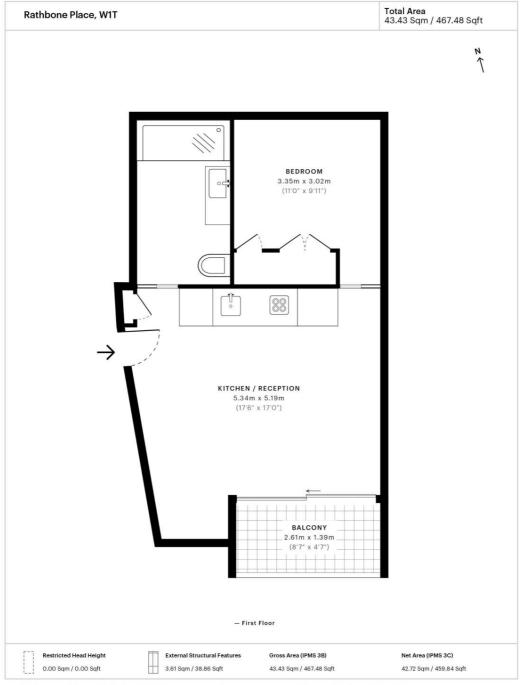
Spec floor plan captured for JLL, Knightsbridge on 17/09/2018 using 28,231,618 laser scan points, accurate to +/- 3cm. Produced in accordance with Royal Institution of Chartered Surveyors Property Measurement Standards, incorporating International Property Measurement Standard (IPMS). If you intend to rely on any measurement in a transaction you should perform your own checks. Plot/Gardens illustrative only and excluded from all area calculations. Specilo: 5b97ca74ed/447365fe497ae
