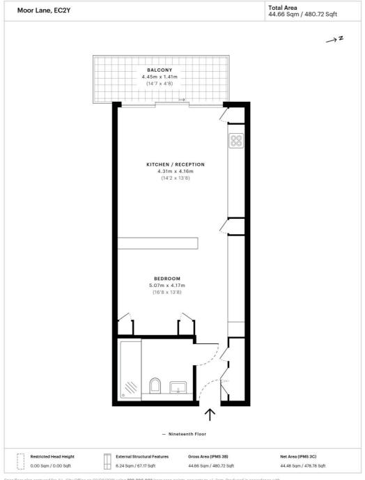
Spec floor plan captured for JLL, City Office on 03/08/2018 using 108,896,982 laser scan points, accurate to +/- 3cm. Produced in accordance with Royal Institution of Chartered Surveyors Property Measurement Standards, incorporating International Property Measurement Standard (IPMS). If you intend to rely on any measurement in a transaction you should perform your own checks. Plot/Gardens illustrative only and excluded from all area calculations. Specilo: 5b630ad6613e220c47d2ef2a
