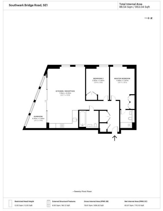
This floor plan was captured for JLL, City Office on 12/06/2018 using 133,967,391 laser scan points, accurate to +/- 3cm and produced in accordance with the Royal Institute of Chartered Surveyors Property Measurement Standards, incorporating International Property Measurement Standard (IPMS). If you intend to rely on any measurement in a transaction you should perform your own checks.
