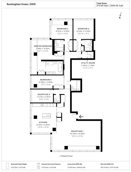
Spec floor plan captured for JLL, Knightsbridge on 03/12/2018 using 79,001,514 laser scan points, accurate to +/- 3cm. Produced in accordance with Royal Institution of Chartered Surveyors Property Measurement Standards, incorporating International Property Measurement Standard (IPMS). If you intend to rely on any measurement in a transaction you should perform your own checks. Plot/Gardens illustrative only and excluded from all area calculations. Specifor 5c013dd81ablad19abd11954
